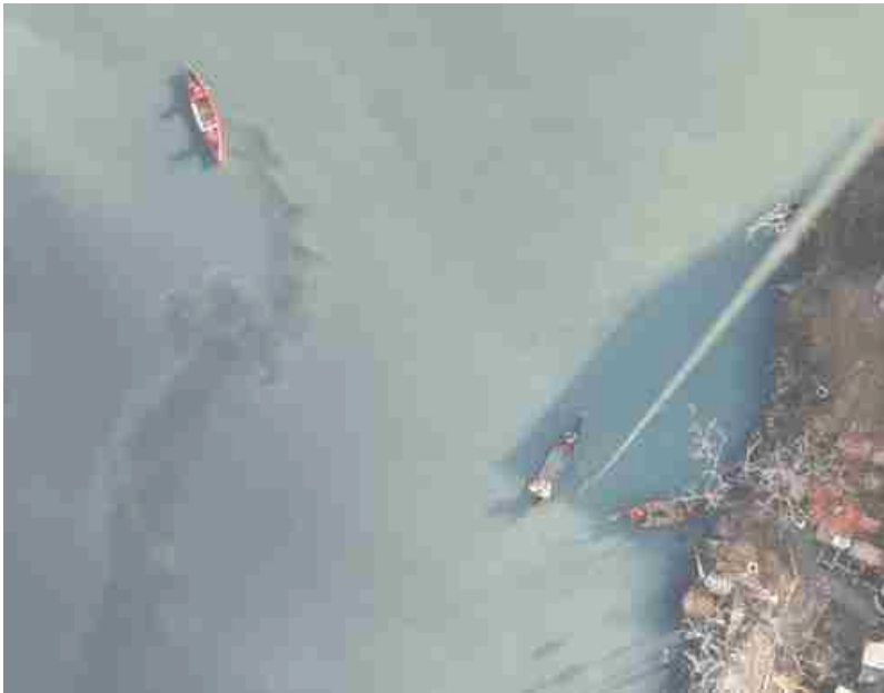
From a Public Lab research note by Eymund Diegal about mapping sewage flows in the Gowanus Canal. Note the people on boats doing the mapping and the balloon tether that links the camera and image back to their bodies.
